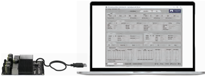
Figure 1: Connect the BVS2300 to a personal computer or laptop and ensure that you have installed the ACP Workbench application.
